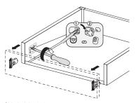
Side height 199 mm (two-step removal)
