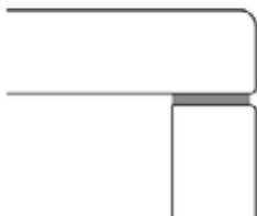
Butt join with shadowline
